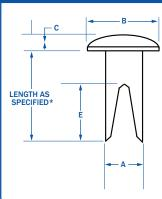
Split rivets are typically used in the luggage, case and leather goods industries to fasten soft materials such as plastics, animal hide and wood. With automatic setting equipment it can pierce through soft materials without a pre-punched hole. Typically offered in Steel or Brass material with a host of metal finishes such as zinc, nickel, or brass plating.
