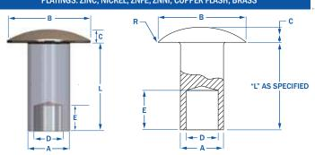
RIVETKING® Semi Tubular Rivets are manufactured in accordance with internal standards and coated with a proprietary wax to insure a smooth rollover and clinch of the assembly.
