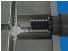
Steel mould, IMTEC® CO and automatic spindle device.
