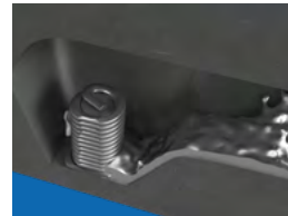
Casting the liquid melted aluminium into the transfer chamber without pressure using dosing machines or manually from a ladle.
