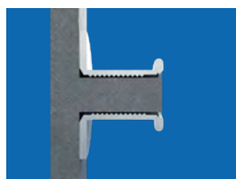
1) Placing on core pin of the injection mould
