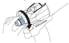
2 Insert the mandrel into the traction bushing.
