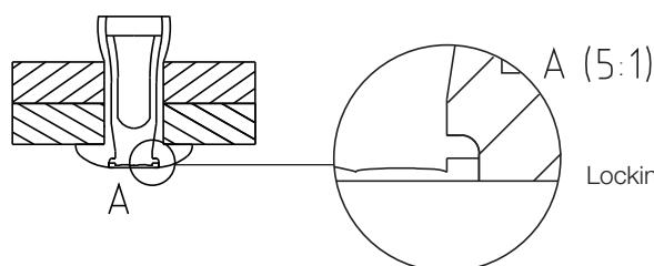
Locking visible after riveting
