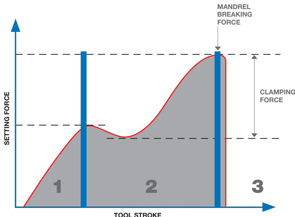
First the rivet is placed in the nose of the setting tool, then it is inserted into the hole and the setting cycle can start. The setting sequence of a blind rivet includes three steps.
