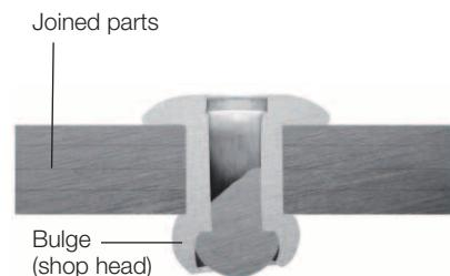
Setting a blind rivet is a simple operation:
