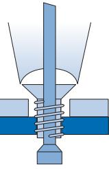
The countersunk head becomes a flat head after riveting
