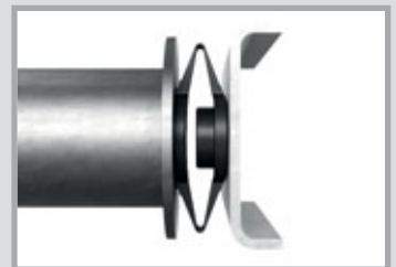
a) Positioning of the components b) Axial tolerance compensation through compression of the FLEXITOL® Eco
