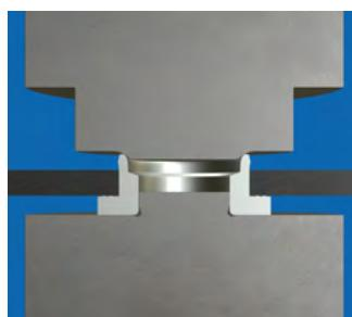
Closing the tool and placing the punch on the shaft end of the KAPTI® Limiter. Start of the forming process.
